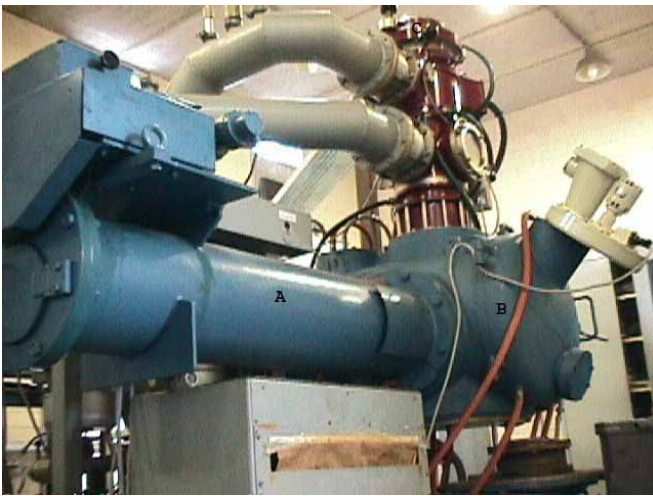
Figure 1. EB furnace, model EMO 80, with 80kW EB power. (A) lateral feeding system; (B) melting chamber and (C) electron gun
