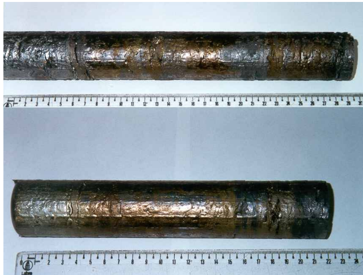
Figure 3. EBM ingot: upper, after first melting; lower, after two remelting.
