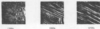
Fig. 1 - Steel BN after rolling at 900°C. The cementite seems lamellar at lower magnification (1300x), but at higher magnification (6700x) the real fibrous structure appears.
