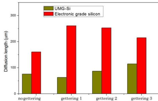
**Figure 3:** Carrier diffusion length of monocrystalline UMG-Si compared to electronic grade silicon (EG-Si)
