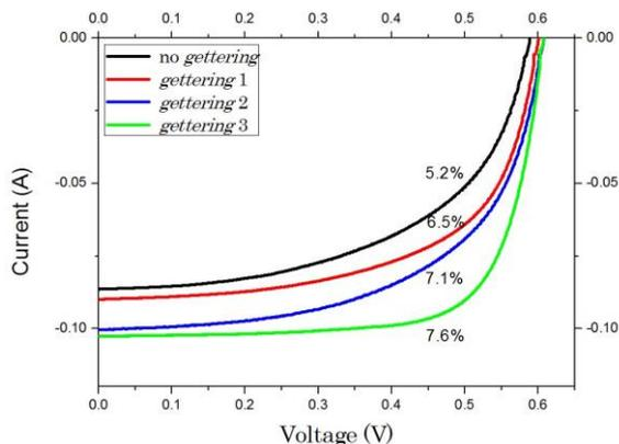
**Figure 2:** Current vs. voltage curves of the best solar cells fabricated with UMG-Si fabricated with different gettering process
