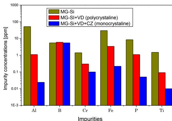
**Figure 1:** Impurity concentration of the silicon feedstock (MG-Si), UMG-Si obtained by vacuum degassing and UMG-Si obtained by a combination of vacuum degassing and CZ
