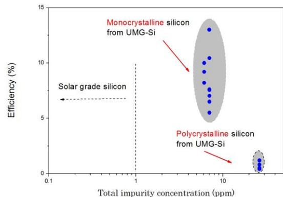
**Figure 4:**Efficiency vs. total impurity concentration of solar cells made with UMG-Si
