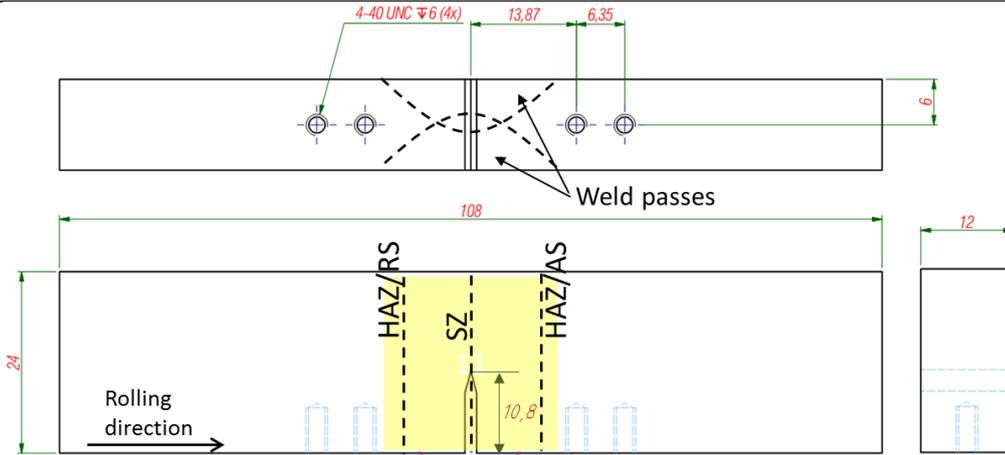
Figure 1. Schematic representation of FSW CTOD single edge notched bend (SENB) specimen with notch located at the stir zone. Notice the plates rolling direction. Dimensions in mm.
