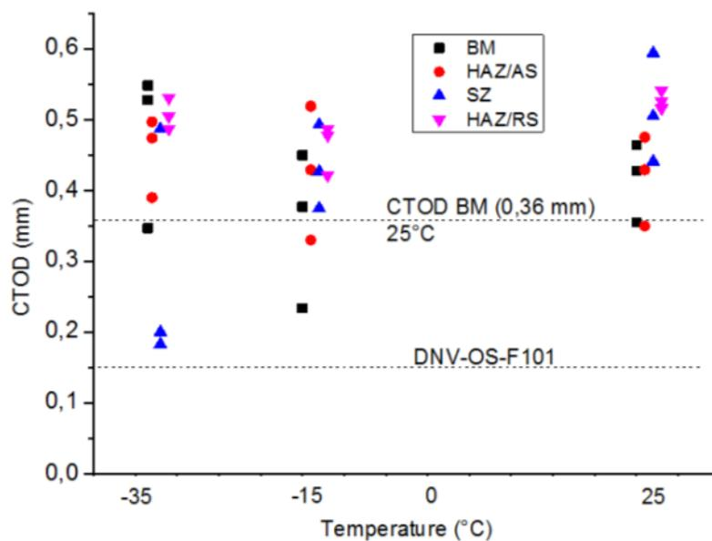
Figure 3.  $CTOD_{cot}$  values for the different FSW regions. BM: Base Material. HAZ/AS: advancing side heat-affected zone, HAZ/RS: retreating side heat-affected zone, and SZ: Stir Zone
