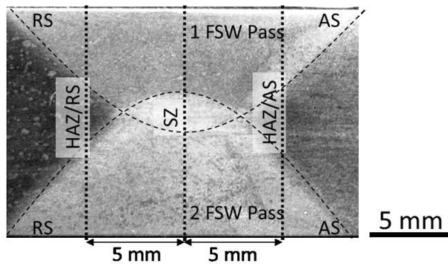
Figure 2. Joint cross section macrograph with the schematic representation of FSW passes and CTOD specimens notches positions.
