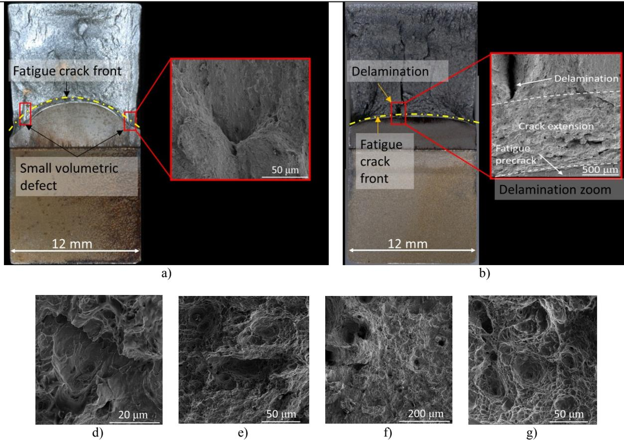
Figure 4. CTOD samples fracture surfaces. a) Weld defect at the advancing side interface has been revealed on the sample tested at 25°C; b) BM fracture surface showing delamination. Stable crack growth region: d) BM; e) SZ; f) HAZ/AS; and h) HAZ/RS.
