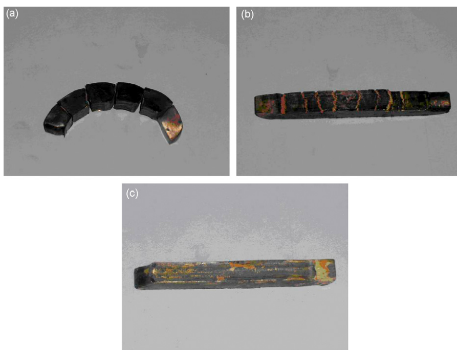
Fig. 2. Appearances of the aluminum bronze billets subjected to ECAE at (a) 550 °C, (b) 600 °C and (c) 650 °C.
