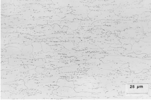
Fig. 7. Microstructure of the tinplate steel in the cold-rolled and annealed condition. Etchant: 2% Nital.
