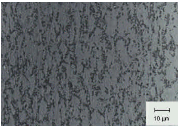
Fig. 4 Micrograph of deformed specimens at 750 °C: v = 0.01 mm/s and e = 62\% .
