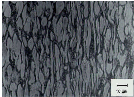
Fig. 3 Micrograph of the initial material as received: longitudinal section.
