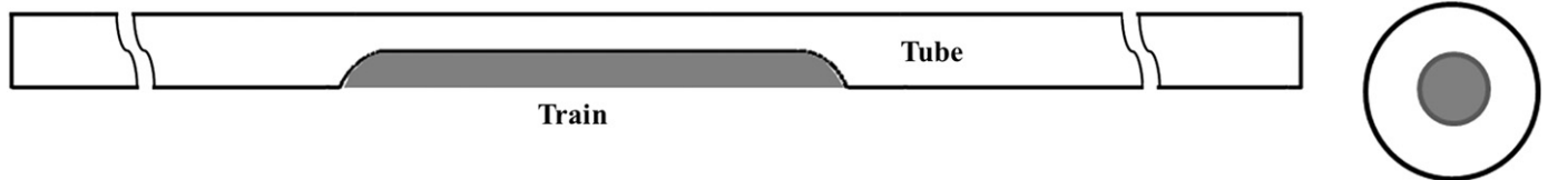
Fig. 1. Schematic of computation domain of tube train system.
