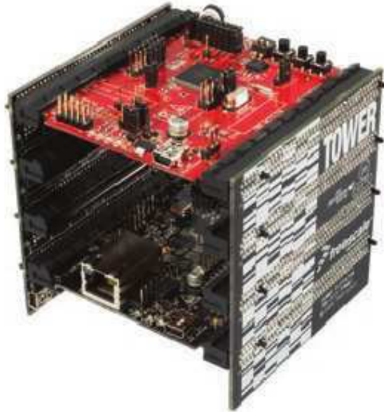
Figura 3.4: TWR-MCF51CN-KIT da Freescale Semiconductor. Fonte: Freescale Semiconductor Inc. (2009b).
