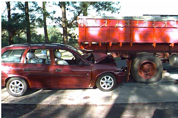
Figure 11 Final position of the car after testing the Brazilian standard guard (constructed according to CONTRAN Regulation No. 805/95 / E.C.E. R 58).
