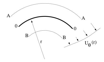
A polar coordinate system  $r - \theta$  with  $\hat{\theta}$  locally aligned with the streamline is introduced. The radial momentum equation degenerates to
