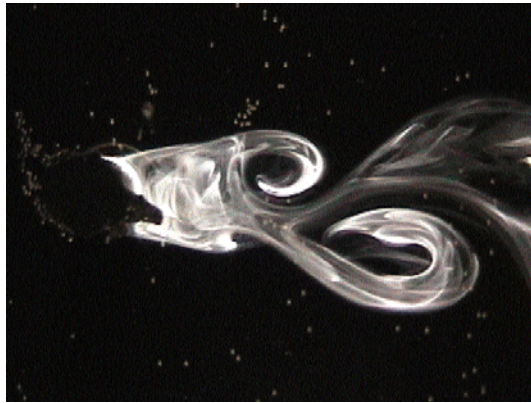
Tin-oxide precipitated in the wake of a cylinder reveals the wake structure. Contributed by Yukie Tanino
