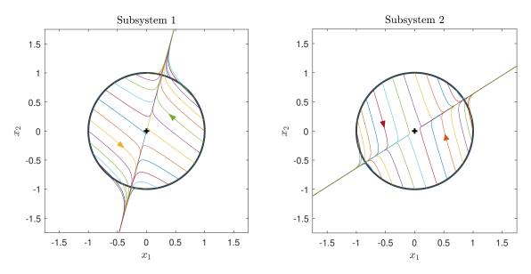
Figure 3.2: Phase portrait for each unforced linear subsystem.
