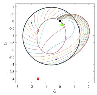
Figure 3.6: Phase portrait for the switched affine system under the min-type quadratic rule.
