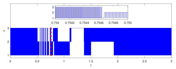
Figure 4.11: Switching rule for the switched affine system under Theorem 4.2.
