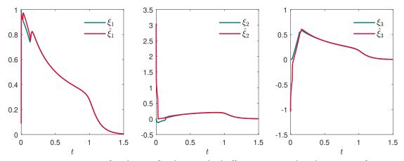
Figure 4.6: Trajectories of each state for the switched affine system under Theorem 4.1 for  $\psi_1$ .
