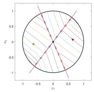
Figure 3.4: Phase portrait for the switched linear system using the min-type quadratic rule.
