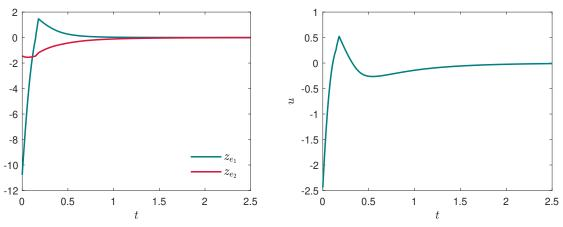
Figure 4.3: Output and control signal for the switched affine system under Theorem 4.1.
