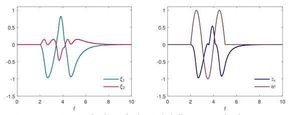
Figure 3.10: Trajectories of each state for the switched affine system under Theorem 3.6.
