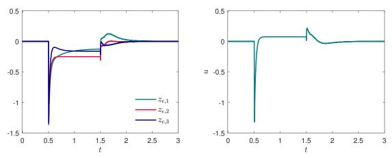
Figure 4.13: Output and control signal for the switched affine system under Theorem 4.3.
