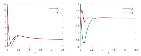
Figure 4.2: Trajectories of each state for the switched affine system under Theorem 4.1.
