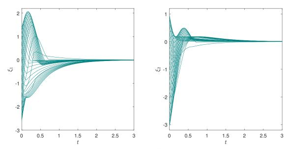
Figure 3.7: Trajectories of each state for the switched affine system under the min-type quadratic rule.
