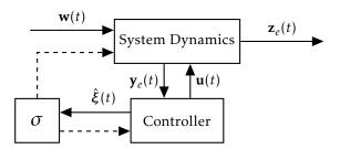
Figure 4.1: Closed-loop system.
