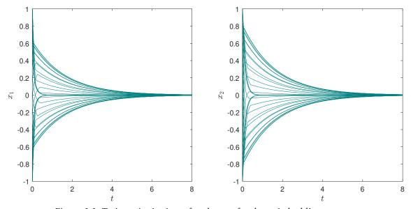
Figure 3.3: Trajectories in time of each state for the switched linear system.
