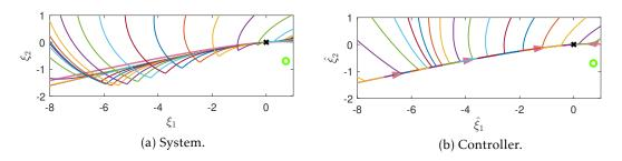
Figure 4.5: Detailed phase portrait for the switched affine system under Theorem 4.1.
