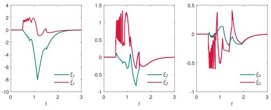
Figure 4.9: Trajectories of each state for the switched affine system under Theorem 4.2.
