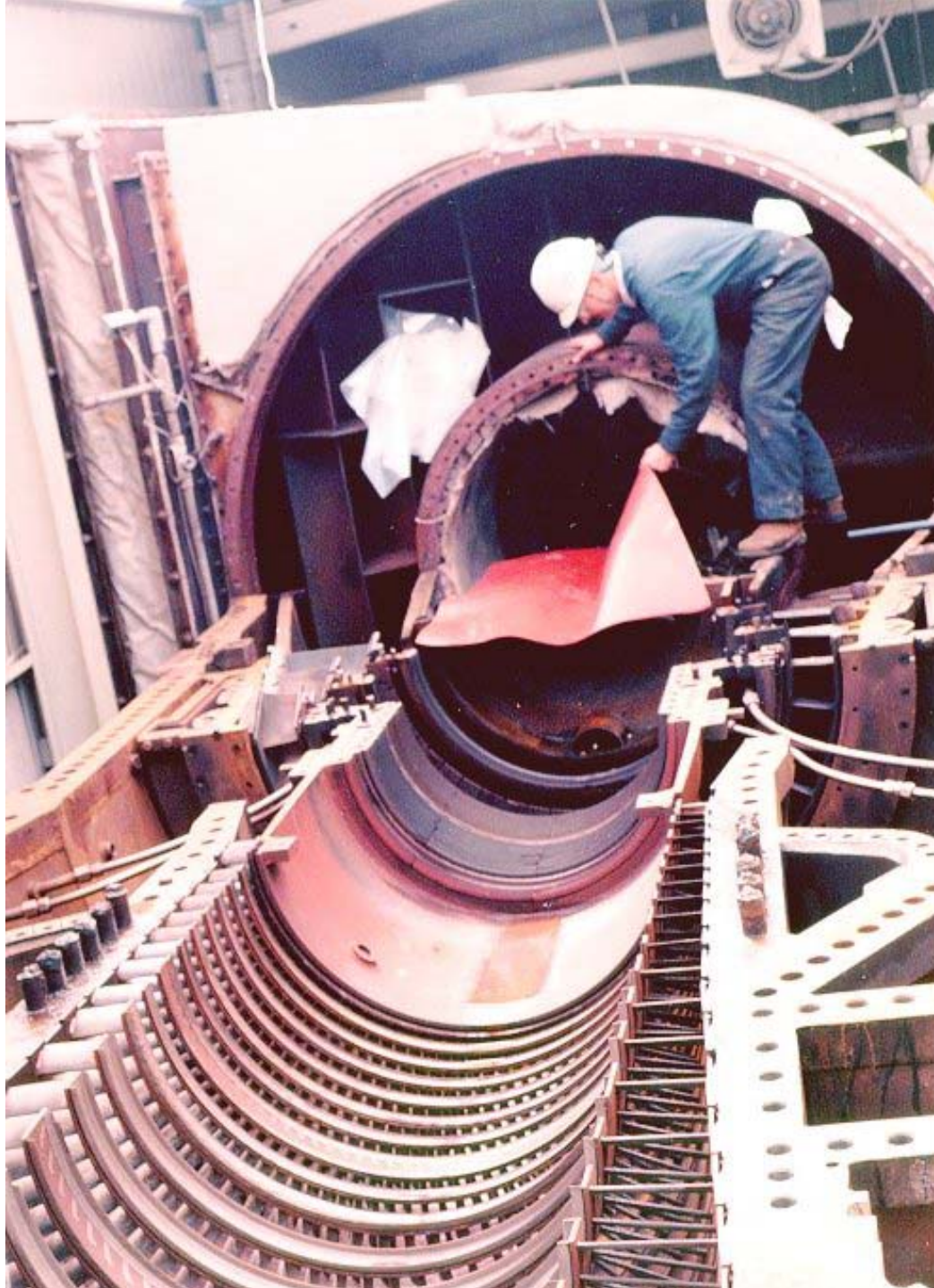
Compressor bed showing compressor stator blades for an industrial gas turbine. (Courtesy of S. Laney)
