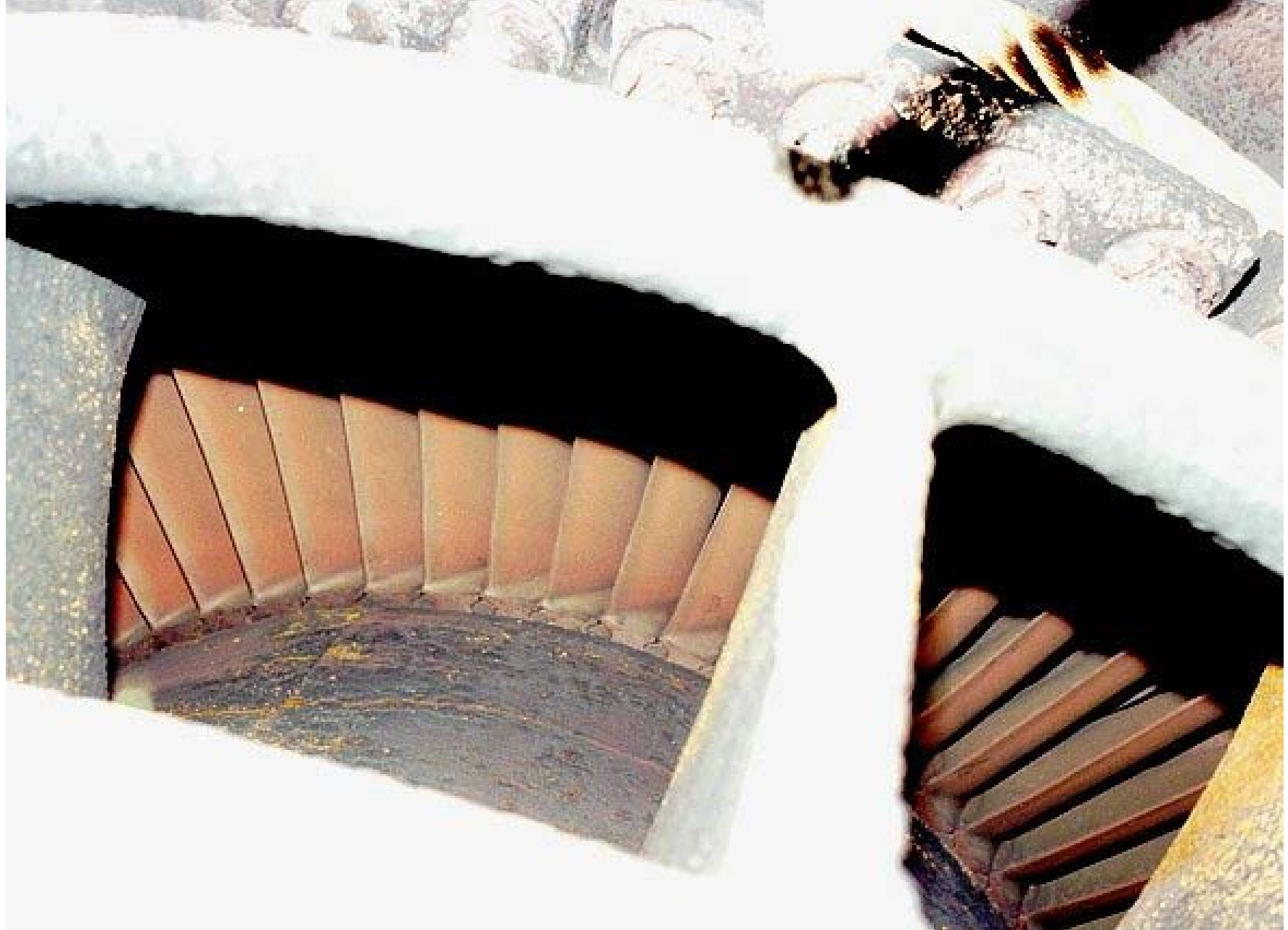
View of power turbine blades in an industrial gas turbine unit. (Courtesy of S. Laney)
