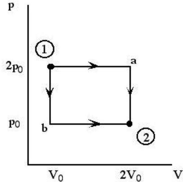
**Question:** Given a piston filled with air, ice, a bunsen burner, and a stack of small weights, describe how you would use these to move along either path a or path b above. When you move along either path how do you physically know the work is different?
