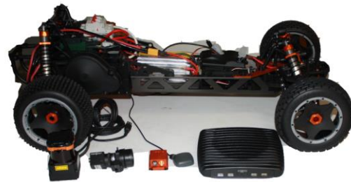
VERDE platform under construction, a mini-Baja vehicle powered by two independent rear motors, a scaled version of the vehicle of VERO Project.
