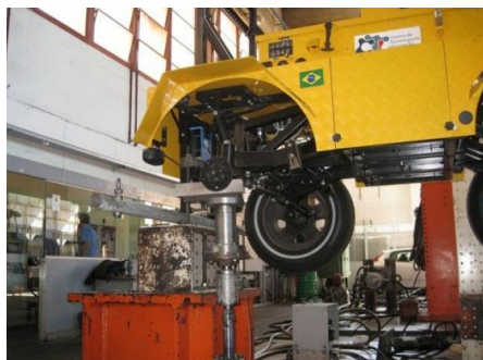
Experimental tests for the validation of the dynamic model used in the VERO simulator, a result of the Master Thesis of Rafael Cordeiro, now in the PhD program under my advisory.
