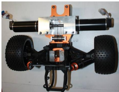
VERDE platform under construction, a mini-Baja vehicle powered by two independent rear motors, a scaled version of the vehicle of VERO Project.
