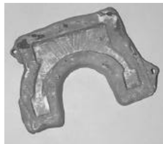
Fig.7 – Forging dies in epoxy: (a) bevel gear, (b) transmission shifter fork.
