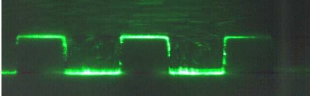
Fig. 6 Flow visualization image obtained for the k-type rough plate. Re = 9.6 \cdot 10^3 .
