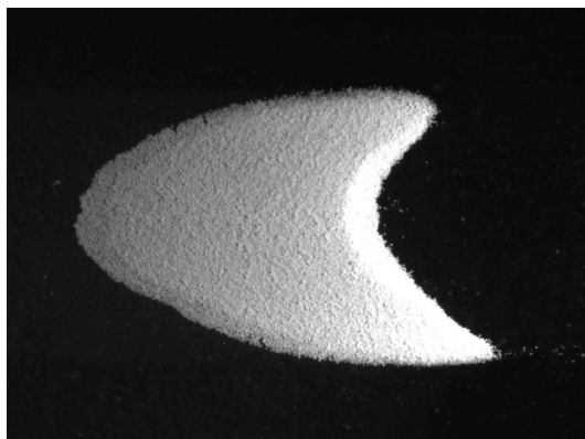
FIGURE 7. Top view of an asymmetric dune with different horn lengths; the dune width is W = 5 cm and the distance to the lateral walls of both horns is the same; the particles leaving the longer horn are clearly visible.
