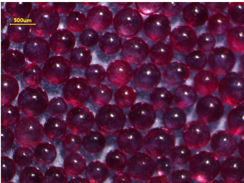
Figure S4. Microscopy image for the 0.40 \text{ mm} \leq d \leq 0.60 \text{ mm} round glass beads of red color.
