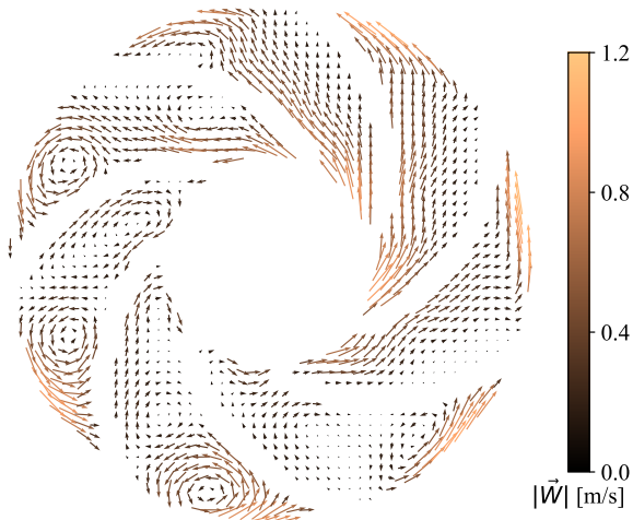
(a) Q_w = 0.1 Q_{BEP} measured next to hub plane
