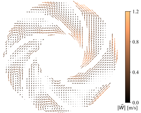
(b) Q_w = 0.1 Q_{BEP} measured next to shroud plane
