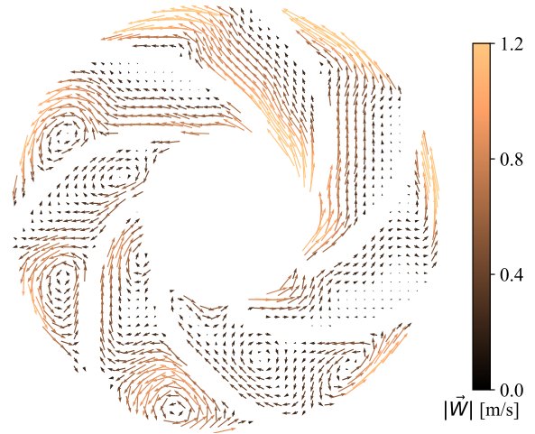
(b) Q_w = 0.1 Q_{BEP} at N = 900 rpm
