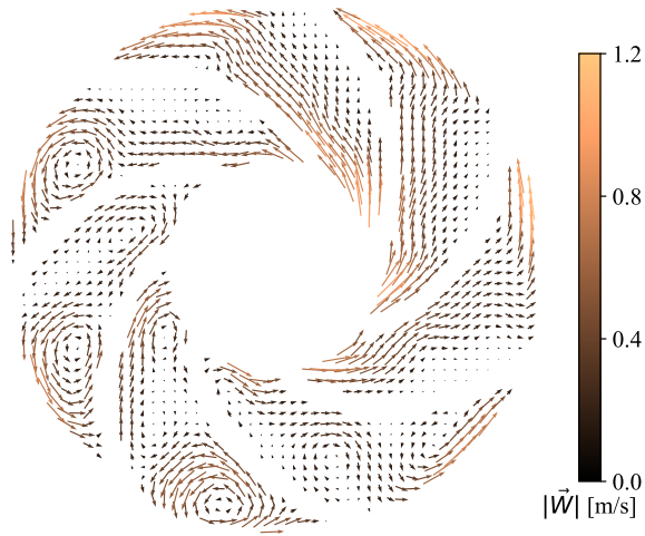
(a) Q_w = 0.1 Q_{BEP} at N = 600 rpm
