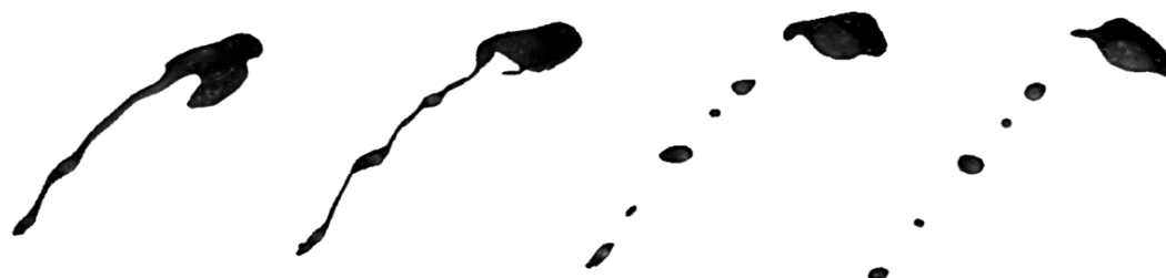
Figure 4. Images of water drops dispersed in mineral oil inside an impeller. As can be seen, one large drop breaks up and originates six smaller drops. Figure adapted from Perissinotto (2018).
