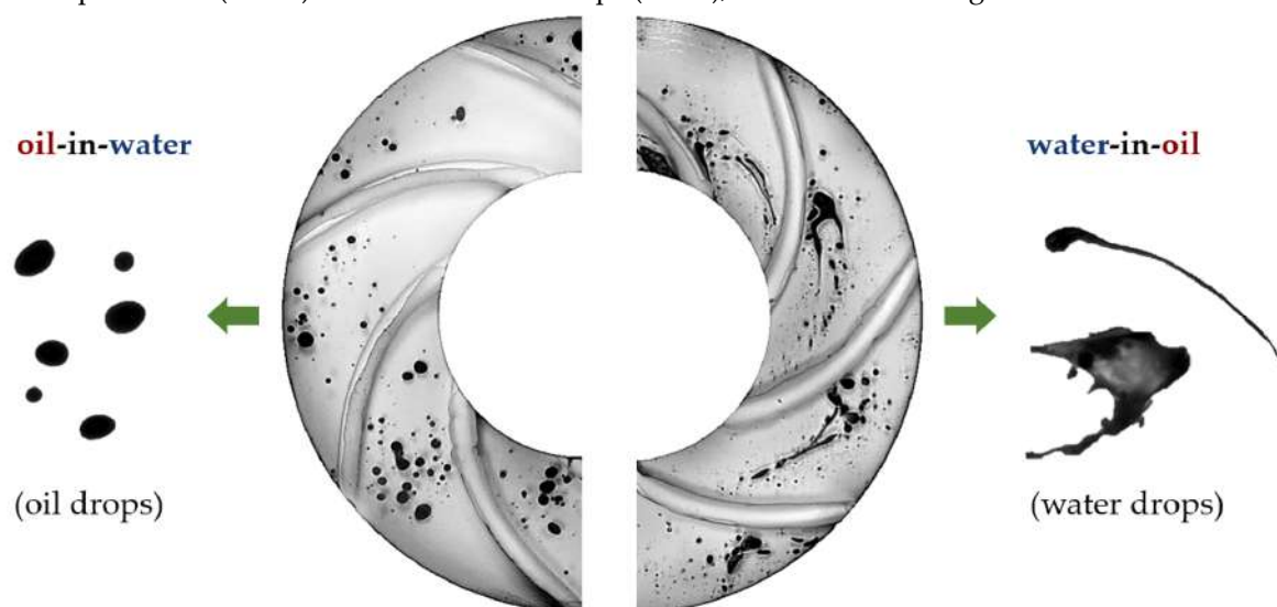
1167 Figure 30. Two-phase liquid-liquid dispersions in the impeller of a transparent prototype rotating at 1168 600 rpm. The continuous phase is transparent and the dispersed phase is darkened with a black dye.
