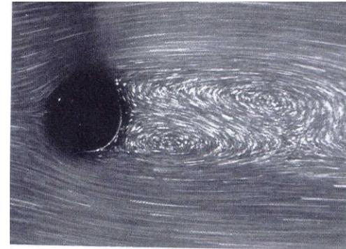
Fig. 3. Flow around a circular cylinder at  $Re = 19$  (water, flow velocity 0.20 cm/s, cylinder diameter 1.0 cm, aluminium powder method and electrolytic precipitation method).
