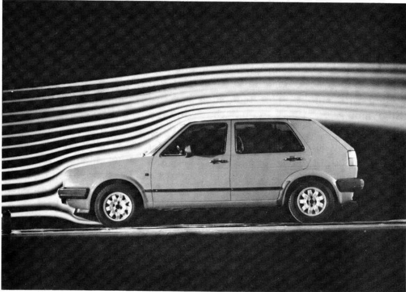
Fig. 2.13 Smoke lines around a road vehicle in a full-scale wind tunnel. (Courtesy of Volkswagenwerk AG.)
