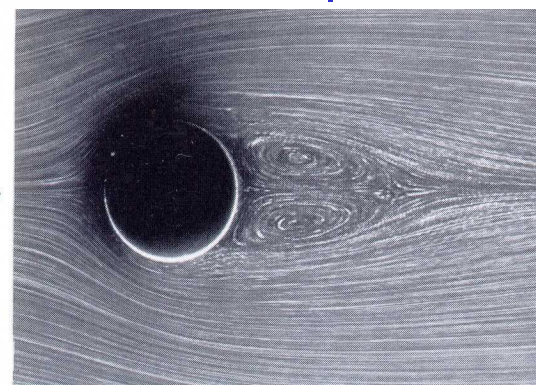
Fig. 4. Flow around a circular cylinder at Re = 26 (water, flow velocity 0.25 cm/s, cylinder diameter 1.0 cm, aluminium powder method).
