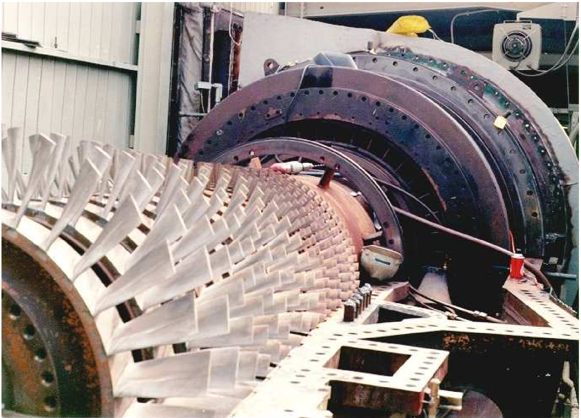
Axial flow compressor for a gas generator unit. (Courtesy of S. Laney)
