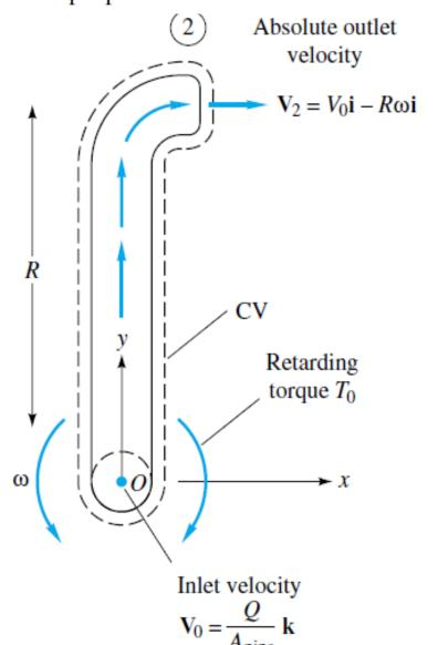
Modify Example 3.14 so that the arm starts from rest and spins up to its final rotation speed. The moment of inertia of the arm about O is  $I_0$ . Neglecting air drag, find  $d\omega/dt$  and integrate to determine the angular velocity  $\omega(t)$ , assuming  $\omega = 0$  at t = 0.
