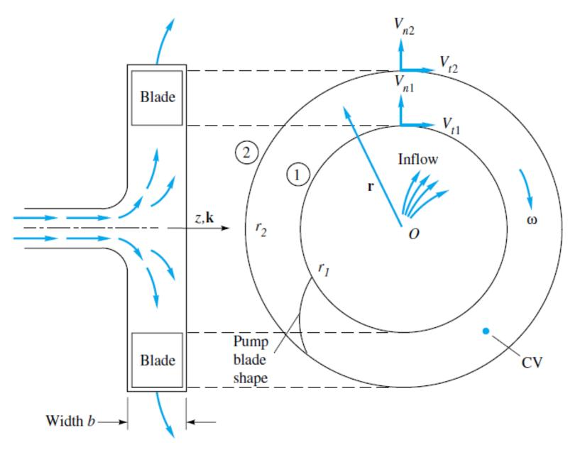
$$T_O = \rho Q \omega (r_2^2 - r_1^2)$$
